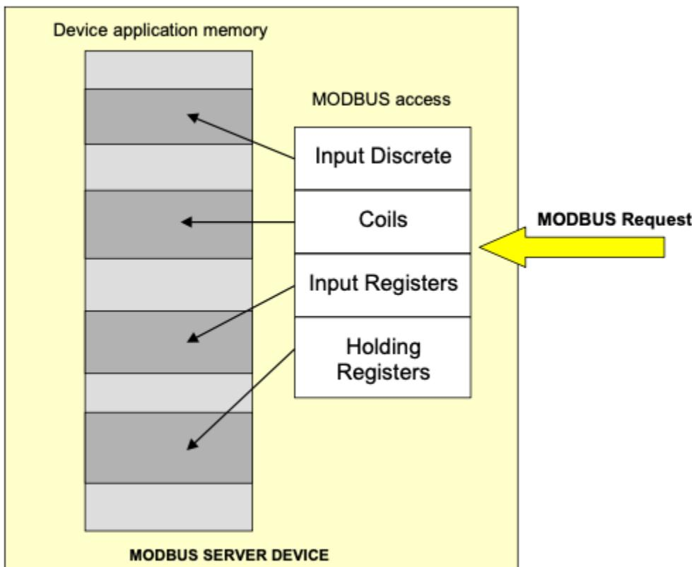
When reading holding register 1 (block 4) you get a different register as when reading input register 1 (block 1). Each block references a different physical register memory, in other words the size of the needed memory is the sum of the block sizes.
