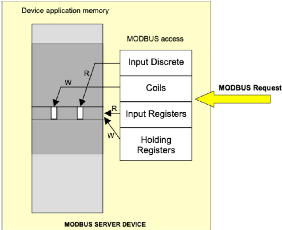
When reading holding register 1 the same physical register is accessed as when reading input register 1. Each block references the same physical register memory, in other words the size of the needed memory is the size of the largest block.
